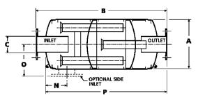
Sizes 11/2" to 31/2" have MNPT connections. Sizes 11/2" through 10" are two chambered. Sizes 12" and larger have three chambers.
